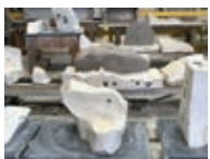
Fig. 30 In-process casting porcelain; deconstructed plaster mold, 2017
